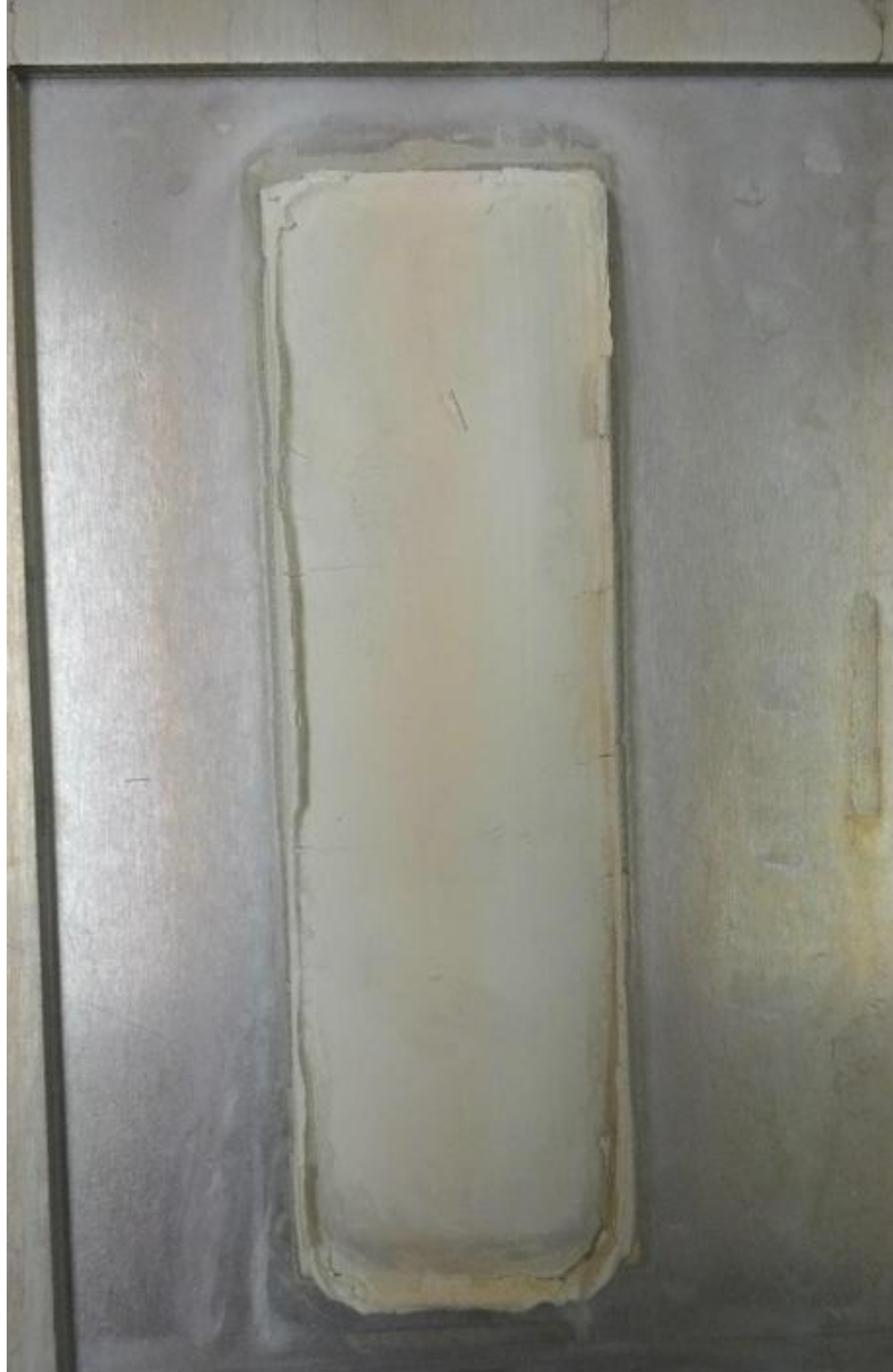
MS sealant QUV test result After >20,000 QUV hours (abt 20 years of actual weather) Observed on 25/10/214, test started 14/05/2012
